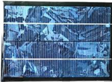
Fig 5 Solar panels producing 6V-300mA.
